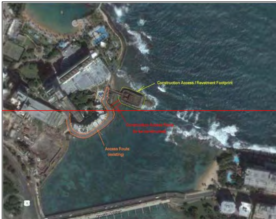
Image 13. Plan View of Revetment and Access Route Footprint
