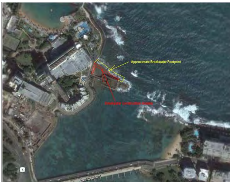
Image 15. Proposed Breakwater Location and Access Ramp View
